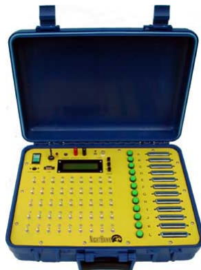
Computer Firing Controls for Demolition Charges
